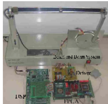
Fig. 7. Experiment setup of the ball and beam system
