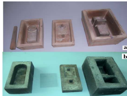
Fig. 1 a) Left to right –sprue, bottom runner core box, top runner core box, pouring basin core box, b) Left to right – Bottom runner core, metal screen, top runner core, pouring basin core
