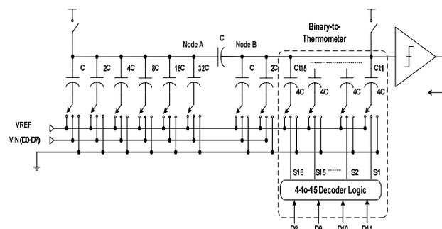
Fig. 1(d) 12-bit with 4-bit thermometer coded DAC
