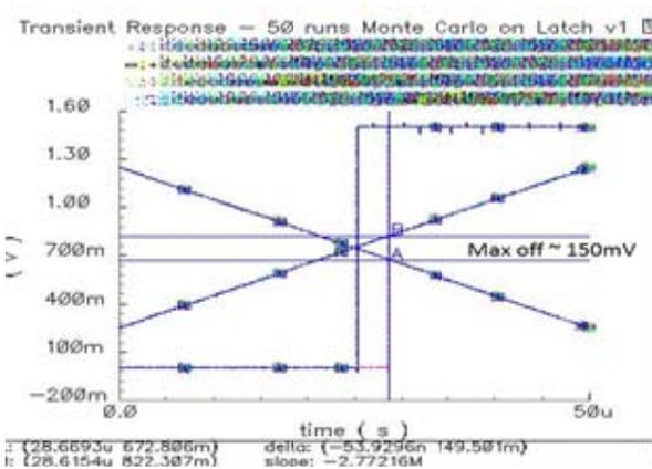
Fig. 4(c) Monte Carlo simulation on Latch circuit
