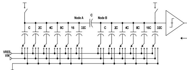
Fig. 1(c) 12-bit DAC with unit value bridge capacitor
