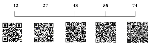
Fig. 4 The quantity of the input characters, respectively in 12,27,43,58 and 72, and their corresponding patterns
