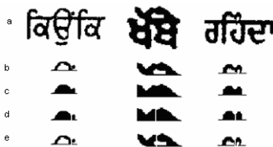
Fig. 18 a) example words, b) problem areas, c) top profile of problem areas, d) segmenting columns in top profiles, e) actual segmented characters
