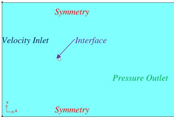
Fig. 7 Boundary conditions of the *Computational Domain sub-grid*
