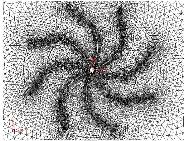
Fig. 8 *Rotor sub-grid* isotropic unstructured mesh
