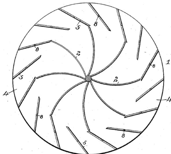
Fig. 3 Horizontal section of the rotor (from: [10])
