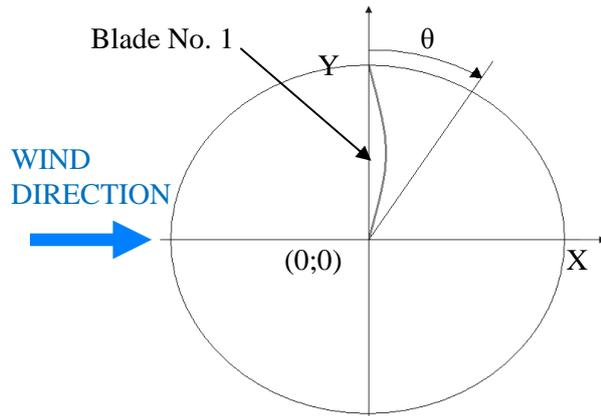
Fig. 6 Azimuthal coordinate of blade No. 1 tip
