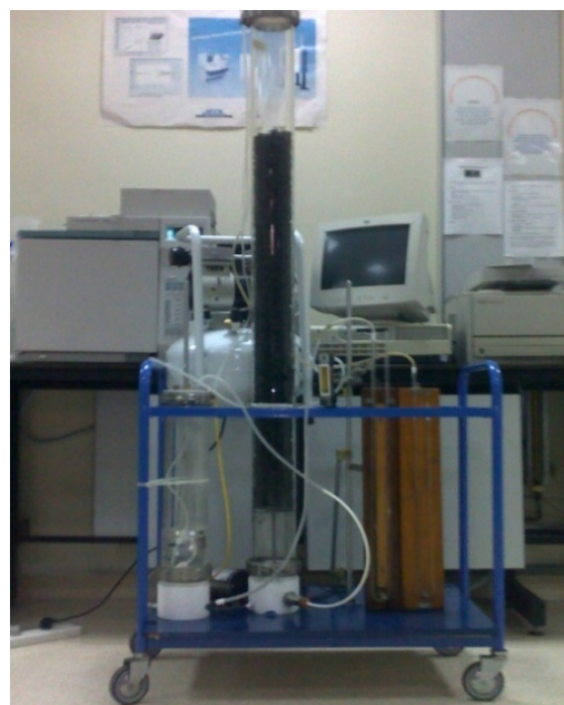
Fig. 3. Photograph of the biofiltration system set-up in the laboratory
