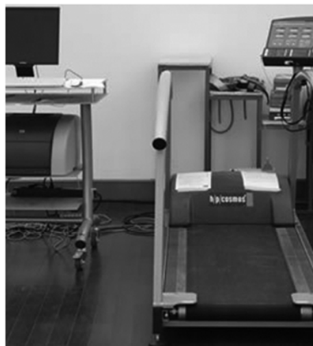
Fig. 1 Treadmill housed with force platform
