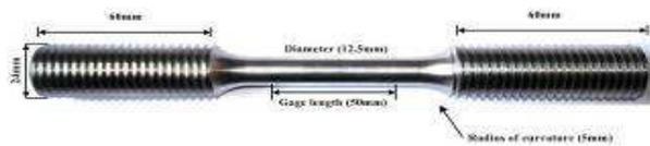
Fig. 2 Test specimen shape and dimension (KS B0801 10)
