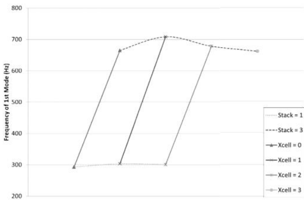
Fig. 12 Variation of frequency of 1st mode for a 3 cell system
