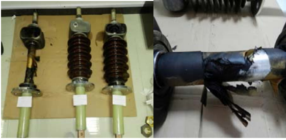
Fig. 1 Photo of three failed transformer bushings
