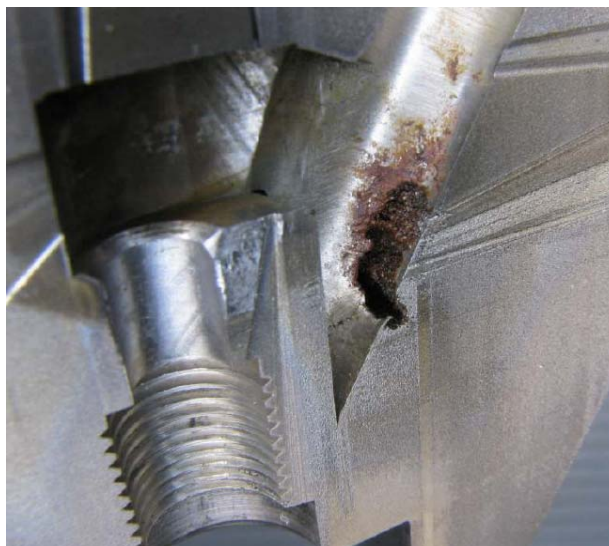
Fig. 9 Cavity found at defect location
