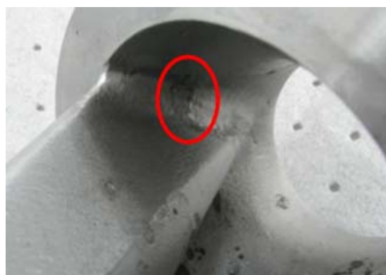
Fig. 4 Suspected casting defect area
