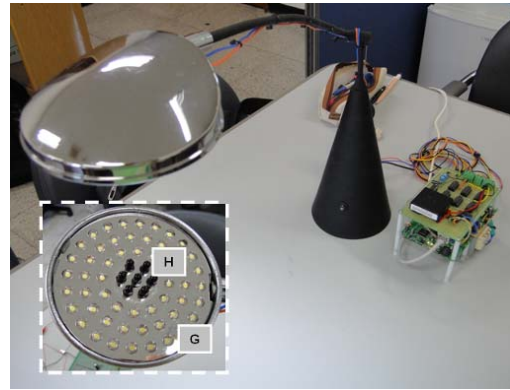
Fig. 4 Photograph of optical transceiver at access point
