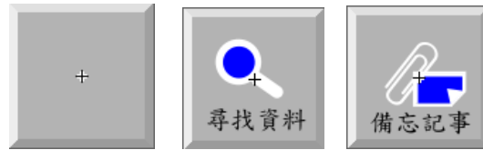
Fig. 1 Design of visual cues (blue region) on touchscreen icons. (a) No cues, control group; (b) TL, the Chinese characters mean "Search"; and (c) BR, the Chinese characters mean "Memo"
