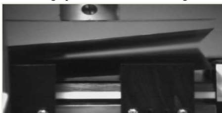
Fig. 7 Wafer lifting during picking process
