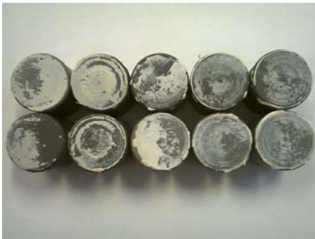
Fig. 6 bonding strength test sample after bond test
