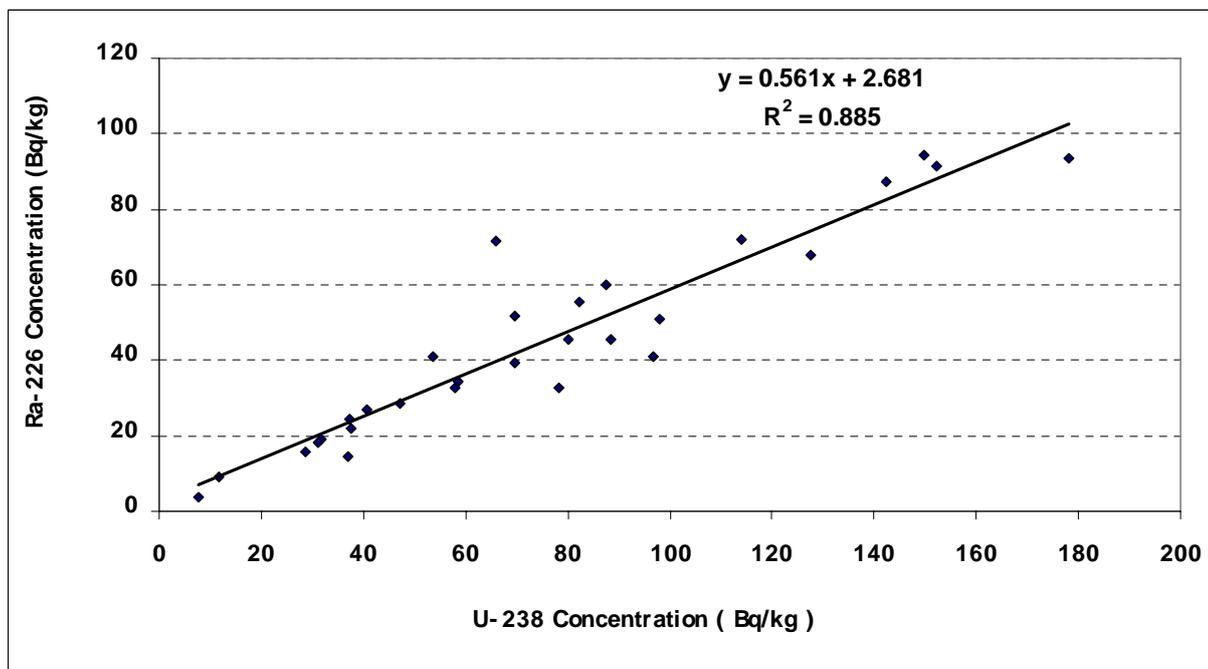
Fig. 4 The correlation between <sup>238</sup>U and <sup>226</sup>Ra concentration in samples
