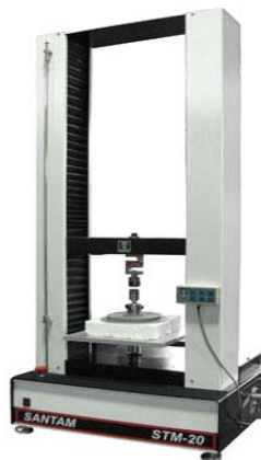
Fig. 1 Apparatus for the measurement of mechanical properties
