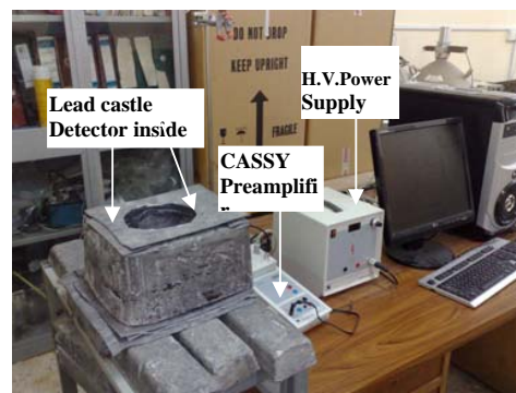
Fig. 2 Physical layout of the NaI(Tl) gamma ray spectroscopy
