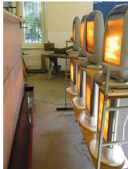
Fig. 3 Warming glass-fiber-concrete façade panel: view to electric warm sources and water tub
