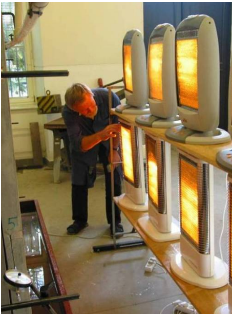
Fig. 15 Warming fiber-cement slab: preparation of equipment
