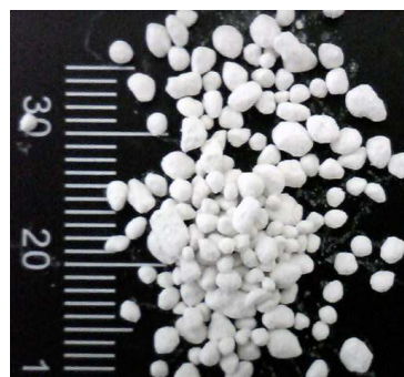
Fig. 1 Granules synthetic Zeolite NaA prepared influid bed metod
