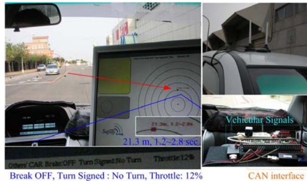
Fig. 16: Remote warning test in short range.
