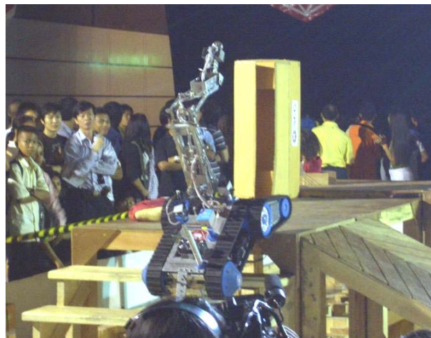
Fig. 1 The CEO Mission II, rescue robot with multi-joint mechanical arm in the Thailand Rescue Robot Championship 2006
