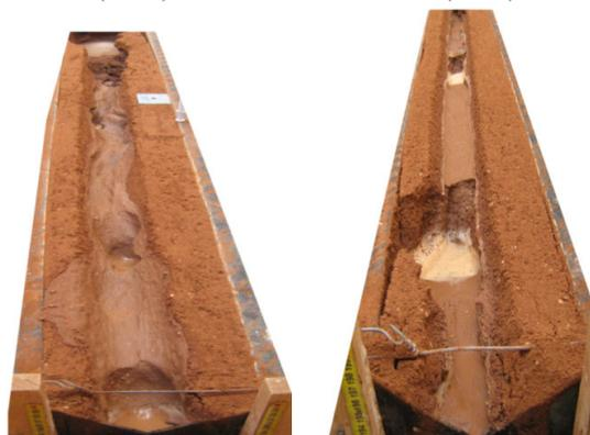
Fig. 4b Types of erosion for circular groove
