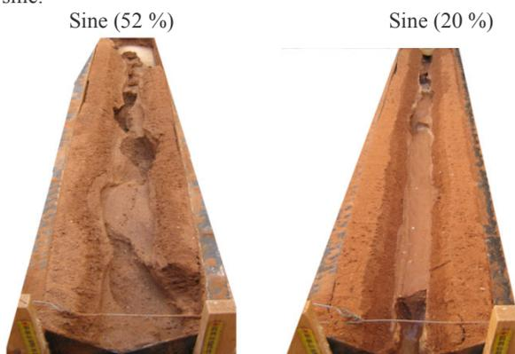
Fig. 4a Types of erosion for sinusoidal groove
