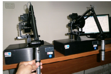
Fig. 7 bilateral teleoperation system using two Phantoms
