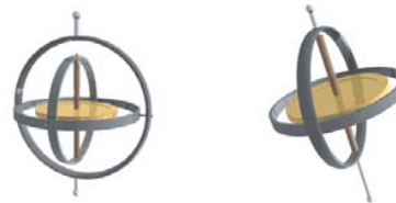
(a) Gimbals set operation (b) Gyroscope frame precession
