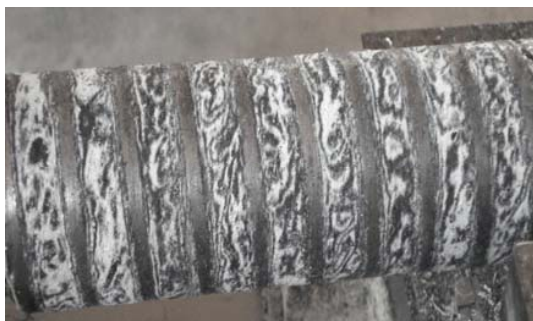
Fig. 3 Fibers wound on the mandrel
