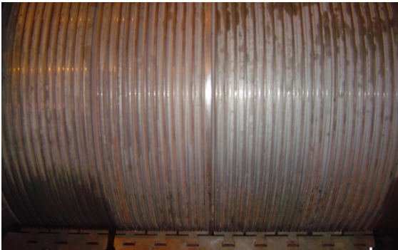
Fig. 1 Effects of rubbing on rotor surface
