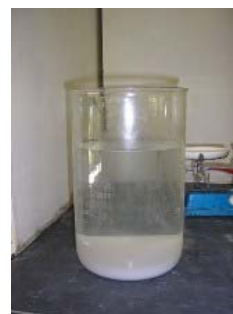
Fig. 6 Lanthanum Oxalate after Three Times Precipitation
