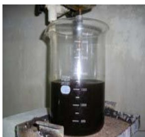
Fig. 4 HNO 3 Digestion of Rare Earth Hydroxide
