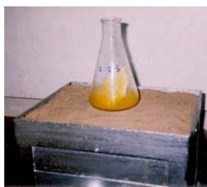
Fig. 2 HCl Dissolution of Hydrous Metal Oxide Cake
