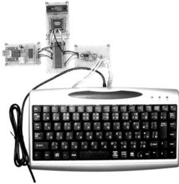
Fig. 2. Prototype of keystroke pressure measurement system with a keyboard.
