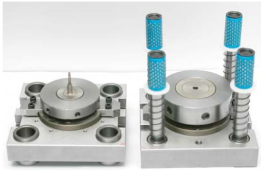
(a) construction of die for micro pattern forming
