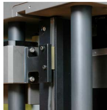
Fig. 5 The linear displacement sensor that have a resolution of 0.1um
