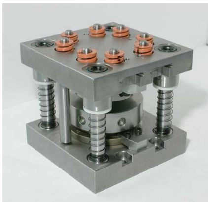
Fig. 7 Die set and spring structure
