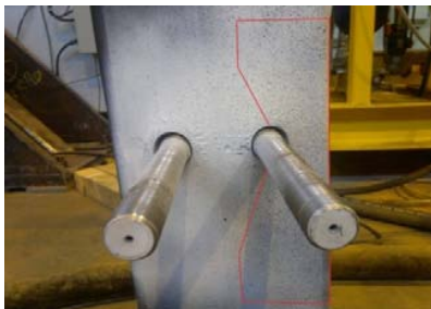
Fig. 7 Area captured by DIC system
