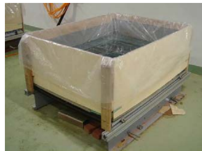
Fig. 4 2400Pa water pressure applied on the module
