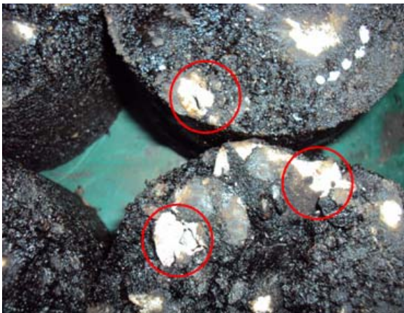
Fig. 4 Broken aggregates during compaction
