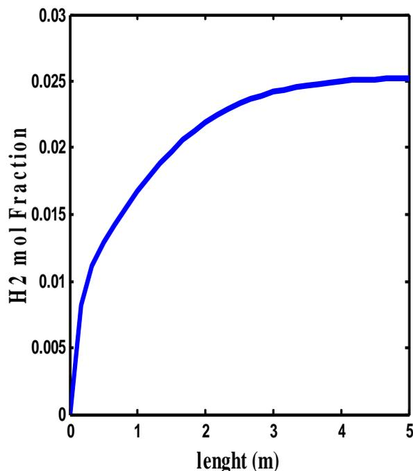
Fig. 5 H<sub>2</sub> concentration profile along the ATR reformer
