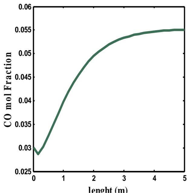
Fig. 4 CO concentration profile along the ATR reformer
