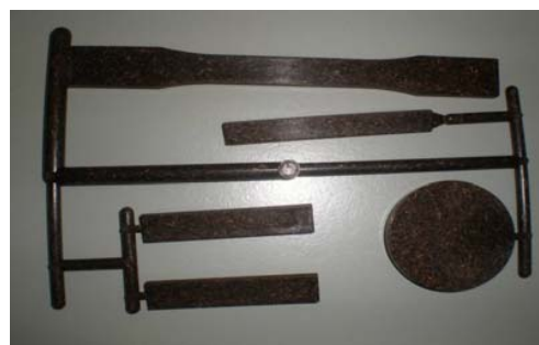
Fig. 1 Photographs of composite samples prepared for tensile, flexural and impact tests
