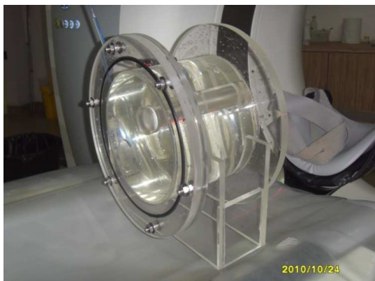
Fig. 1 The setup for phantom scanning in CT scanner
