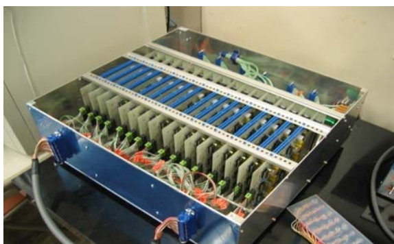
Fig. 4 A 96 channels SEMG amplifier
