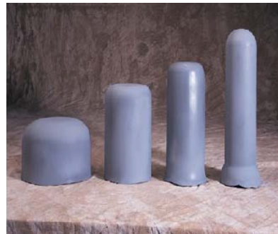
Fig. 3 Specimen that have been successfully drawn
