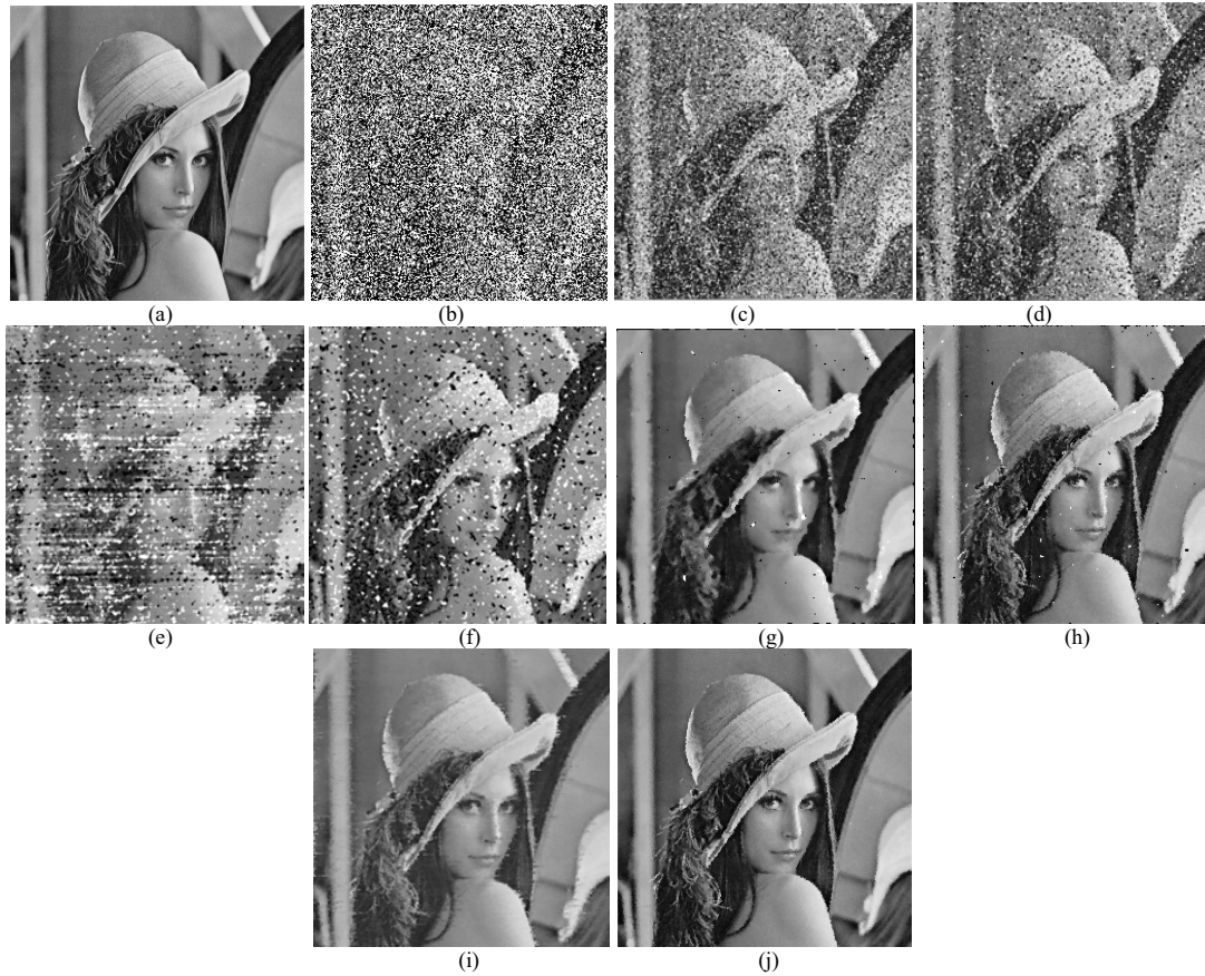
Fig. 6 (a) Original Lena image (b) Noisy image of noise density 70%. Restoration results of (c) Standard median filter (d) Weighted median filter (e) Recursive weighted median filter (f) SD-ROM (g) Progressive switching median filter (h) Adaptive median filter (i) Decision based algorithm (j) Proposed method
