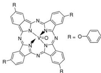
**Fig. 1:** Molecular structure of VOPc.
