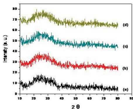
**Fig. 4:** X-ray diffraction patterns of VOPc thin films spin coated on glass substrates: (a) pristine and annealed at (b)  $95^{\circ}\text{C}$ , (c)  $125^{\circ}\text{C}$  and (d)  $155^{\circ}\text{C}$ .
