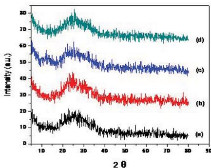
**Fig. 5:** X-ray diffraction patterns of VOPc thin films thermally deposited on glass substrates: (a) pristine and annealed at (b)  $95^{\circ}\text{C}$ , (c)  $125^{\circ}\text{C}$  and (d)  $155^{\circ}\text{C}$ .
