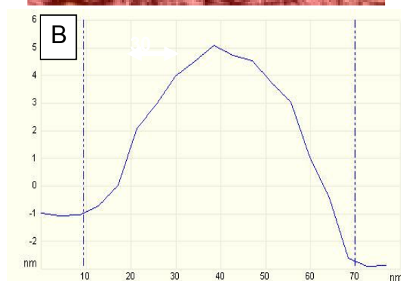
Fig. 3 3D AFM image of the developed Q2D \text{Nb}_2\text{O}_5 nano-sheets deposited on quartz A with height measurements B
