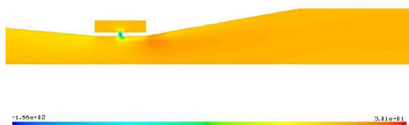
Fig. 8 Contour of velocity in perpendicular to flow direction in 12-holes mixer (m/s)
