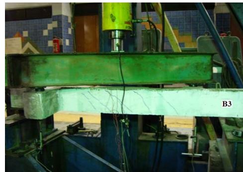
Fig. 4 (d) Failure modes and crack patterns of the tested beam B3
