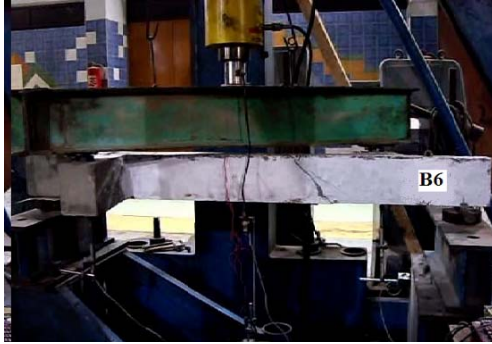
Fig. 4 (g) Failure modes and crack patterns of the tested beam B6
