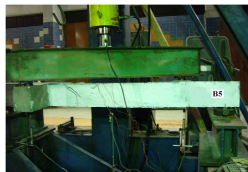
Fig. 4 (f) Failure modes and crack patterns of the tested beam B5
