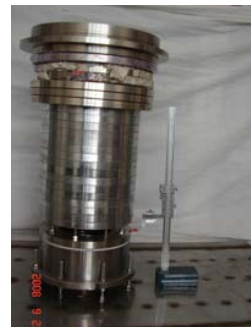
Fig. 5 Test Device of the Pulling Force Measurement
