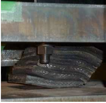
Fig. 6 Deformed STRP-6 at 103% lateral deformation
