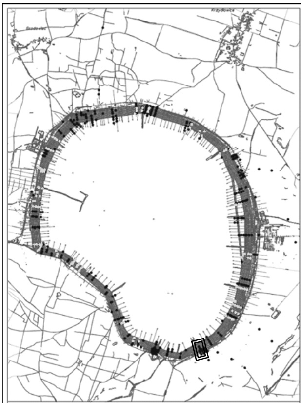
Fig. 3 Plan view of the Zelazny Most tailing dam – the black dots show the locations of the CPTs performed and the light grey dots show the locations of the CPTs used in further analysis
