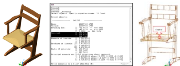
Fig. 6 Analysis for center of gravity using computer aided engineering (CAE)
