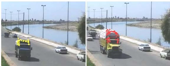
Fig. 4 Result of first test, an over-height vehicle detection (over 2.5 meters)
