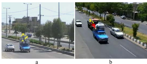
Fig. 6 a. Result of second test, an over-height vehicle detection (over 2.5 meters) b. Result of third test, an over-height (2.5 meter) detection in occlusion situation
