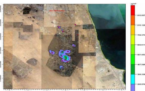
Fig. 3b Isoleths plot for the maximum daily average ground level concentrations of non-methane hydrocarbons in \mu\text{g}/\text{m}^3
